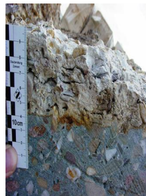
Biogenic sulphuric acid corrosion of concrete – aggressive, fast proceeding decrease .
