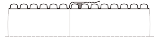
SAFECONNEC®: Inline bellings with reinforcement tape
